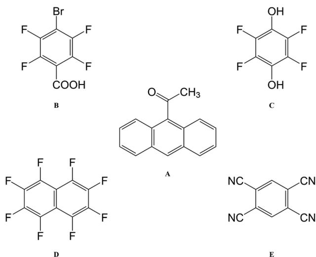
**Fig. 2** Molecular structures of 9-acetylanthracene (A) and its four cofromers: 4-bromotetrafluorobenzenecarboxylic acid (B); 2,3,5,6-tetrafluorohydroquinone (C); octafluoro-naphthalene (D); and 1,2,4,5-tetracyanobenzene (E).
