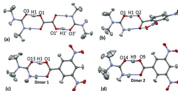
Fig. 3 The carboxylic acid:amide  $R_2^2(8)$  hydrogen bonded dimers in the multipole refined crystal structures with respective H-atom models implemented of (a) 1, (b) 2, (c) 3 dimer 1 (3d1) and (d) 3 dimer 2 (3d2) at 100 K. The oxalic acid molecule in 1 occupies an inversion centre through the central C—C bond and thus the symmetry related portion is shown for completeness.
