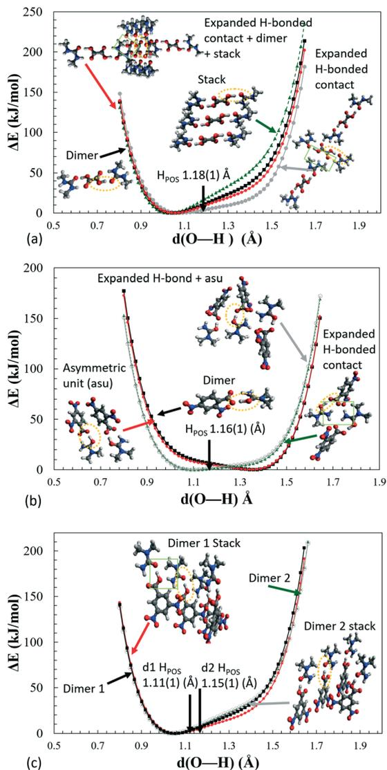
**Fig. 8** H-Atom potentials *in vacuo* of various 'cluster' models of (a) **1**, (b) **2** and (c) **3**, where the proton on the central dimer highlighted by an ellipse (yellow) is moved by 0.02 Å increments between the donor and acceptor oxygens. The green box highlights the presence of extra H-bonding in the expanded H-bonding model. The H-atom position as found in the crystal structure is indicated by black arrows ( $H_{\text{POS}}$ ).
