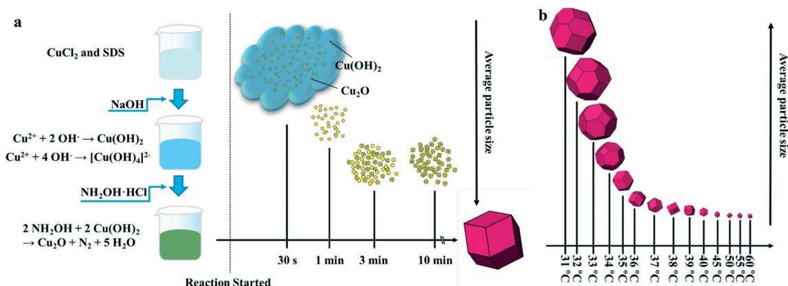
Fig. 1 (a) Schematic diagram of particle size and morphology evolution of d-Cu<sub>2</sub>O with increasing reaction time synthesized at a specific temperature. (b) Schematic diagram of particle size and morphology evolution of d-Cu<sub>2</sub>O with increasing synthesis temperature.
