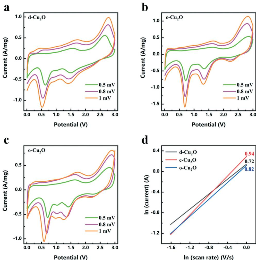
Fig. 8 CV curves of (a) d-Cu<sub>2</sub>O, (b) c-Cu<sub>2</sub>O, and (c) o-Cu<sub>2</sub>O measured at different scanning rates from 0.5 to 1 mV s<sup>-1</sup> after activation at 0.2 mV s<sup>-1</sup> for three cycles. (d) Relationships between ln(current) and ln(scan rate) for d-Cu<sub>2</sub>O, c-Cu<sub>2</sub>O and o-Cu<sub>2</sub>O (peaks of potential at 2.5–3 V).
