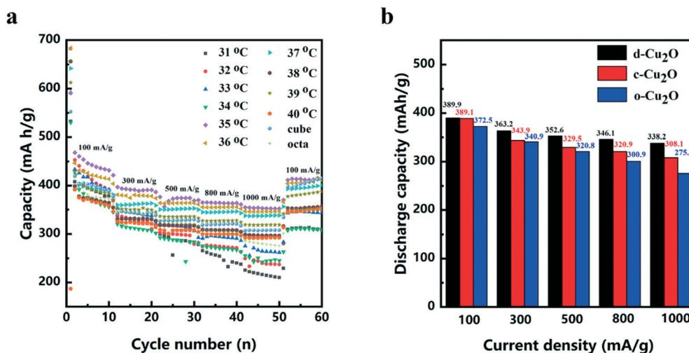
Fig. 7 (a) High rate cycling performance of d-Cu<sub>2</sub>O (reaction temperatures from 31 to 40 °C), c-Cu<sub>2</sub>O and o-Cu<sub>2</sub>O. (b) Discharge capacity of d-Cu<sub>2</sub>O (synthesized at 37 °C), c-Cu<sub>2</sub>O and o-Cu<sub>2</sub>O with the current density ranging from 100 to 1000 mA g<sup>-1</sup>.
