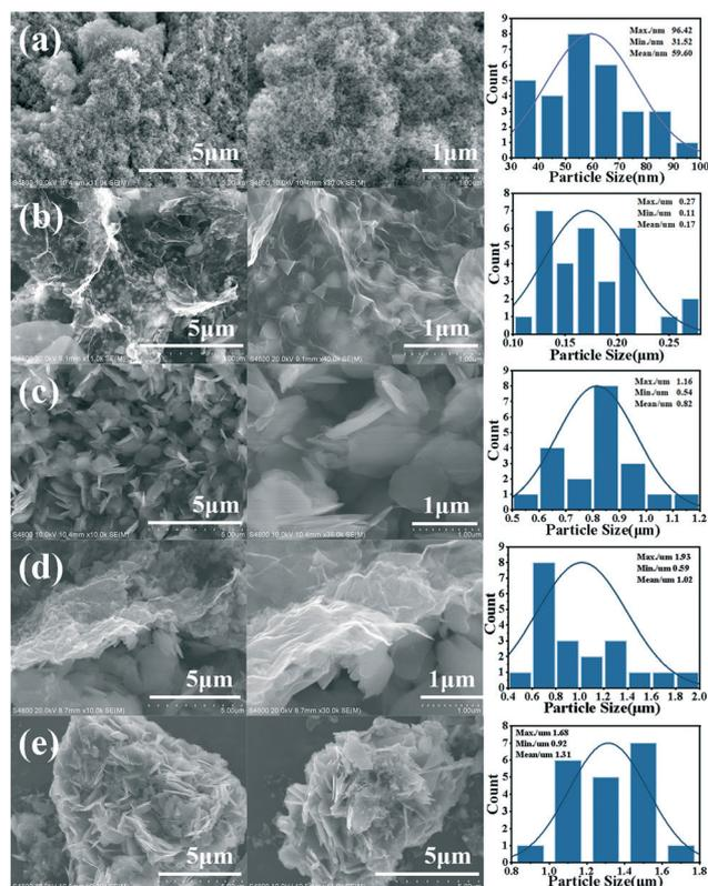
Fig. 2 SEM images and particle size distribution diagrams of pristine  $\text{Co}_3\text{O}_4$  (a) and g- $\text{Co}(\text{OH})_2$  with different hydrothermal reaction times: (b) 3 h; (c) 6 h; (d) 9 h and (e) 12 h.
