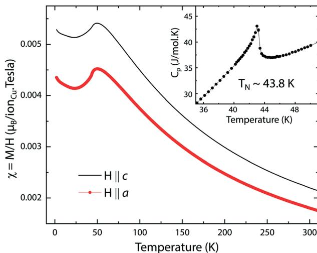
**Fig. 8** Temperature dependence of the magnetic susceptibility  $\chi(T)$  in a magnetic field of 1 T applied along two perpendicular directions, along the  $c$  and  $a$  axes in  $\text{Bi}_2\text{CuO}_4$ , respectively. The inset shows the  $a$ -like specific heat anomaly associated with the antiferromagnetic ordering at  $T_N \sim 43.8$  K.
