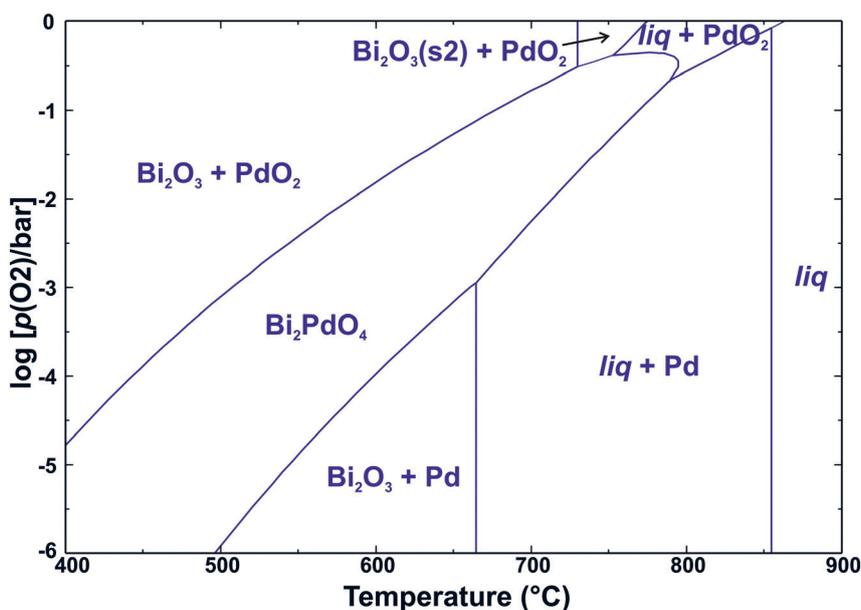
Fig. 6 Phase stability in the system Bi–Pd– $\text{O}_2$ . An enthalpy of 20  $\text{kJ mol}^{-1}$  was assumed for the reaction  $\text{Bi}_2\text{O}_3 + \text{PdO} \rightarrow \text{Bi}_2\text{PdO}_4$ .
