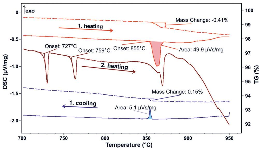
Fig. 2 Bi<sub>2</sub>CuO<sub>4</sub> single crystal TG–DSC measurement (1st and 2nd heating + 1st cooling at 5 K min<sup>-1</sup>) in flowing 66.7% O<sub>2</sub> + 33.3% Ar. Solid lines: DSC, dashed lines: TG.
