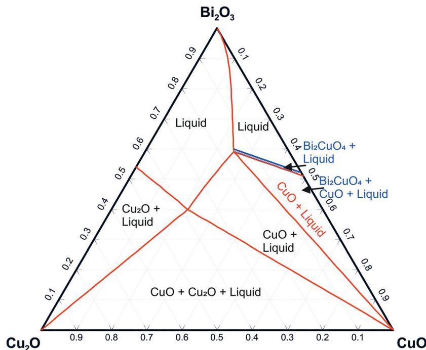
Fig. 4 Isothermal sections through the  $\text{Bi}_2\text{O}_3$ - $\text{Cu}_2\text{O}$ - $\text{CuO}$  system above (857 °C, red) and below (856 °C, blue) the peritectic temperature where  $\text{Bi}_2\text{CuO}_4$  decomposes.
