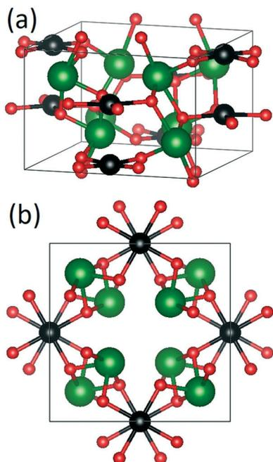
Fig. 1 (a) 3D tetragonal crystal structure of  $\text{Bi}_2\text{MO}_4$  and (b) projection along the  $c$ -axis (green = Bi, black = Cu/Pd, red = O) (drawn with VESTA<sup>30</sup>).
