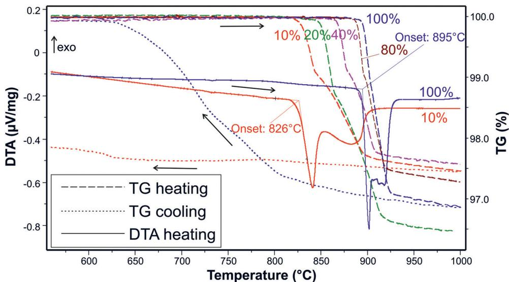
Fig. 5 TG heating curves of  $\text{Bi}_2\text{PdO}_4$  in five different atmospheres from 100%  $\text{O}_2$  to 10%  $\text{O}_2$  in Ar ( $\text{O}_2$  concentration given as a parameter). For the measurements at 100% (blue) and 10%  $\text{O}_2$  (red), DTA heating and TG cooling curves are shown additionally.
