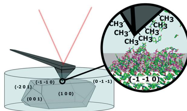
**Fig. 1** Schematic of the experimental setup with a paracetamol crystal mounted in an atomic force microscopy (AFM) liquid cell. In the right part of this schematic, the probe is approaching a dynamic heterogeneous disordered surface (DHDS) layer, indicated in grey colour, on the  $(-1-1\ 0)$  surface of paracetamol in water–ethanol mixture.
