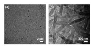
**Fig. 4** TEM images of **1a** prepared from a DMSO solution (a) before and (b) after UV irradiation.
