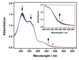
Fig. 3 UV-Vis absorption spectral traces of **1a** in DMSO solution at 298 K upon prolonged UV irradiation at 310 nm for 20 hours. Inset: Magnified UV-vis absorption spectral traces in the low-energy absorption region. The asterisk denotes an instrumental artifact. The direction of arrows indicates the direction of spectral changes upon UV irradiation.
