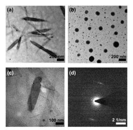
Fig. 2 TEM images of (a) 1a and (b) 2a prepared from a 50% DMSO-water mixture. (c) Magnified TEM image of 1a and (d) the corresponding SAED
