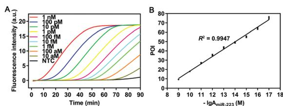
Fig. 2 Sensitivity and dynamic range of the SqPIA assay. (A) Real-time fluorescence curves of miR-223 at nine different concentrations ranging from 10 aM to 1 nM, and the group without miR-223 was considered as the negative control simultaneously. (B) Linear relationship between POI values and negative logarithmic values of concentration. Error bars represent the SD of three independent replicates.
