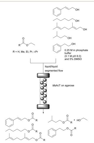
**Fig. 7** Continuous *Ms*AcT catalysed transesterification of primary alcohols in a biphasic system with segmented flow.
