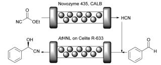
Fig. 3 Two-step synthesis of (R)-mandelonitrile catalysed by CALB and AtHNL.
