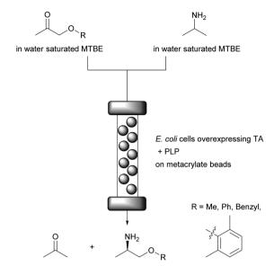
**Fig. 10** Stereoselective amine synthesis catalysed by immobilised *E. coli* cells and PLP on metacrylate beads.
