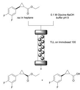
Fig. 5 TLL catalysed kinetic resolution of rac-cyclopropanecarboxylate ester yielding (15,25)-2-(3,4-difluorophenyl) cyclopropan-1-acid. The unaltered (1R,2R) ester is converted into the desired amine.
