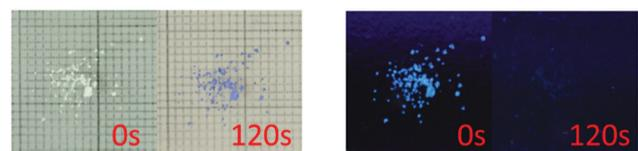
Fig. 4 Powder form of carborane photoswitch **2** taken under white light (right) and UV light (left). The length of time taken in seconds after UV irradiation ( $0.96 \text{ mW cm}^{-2}$ , 302 nm) are given.
