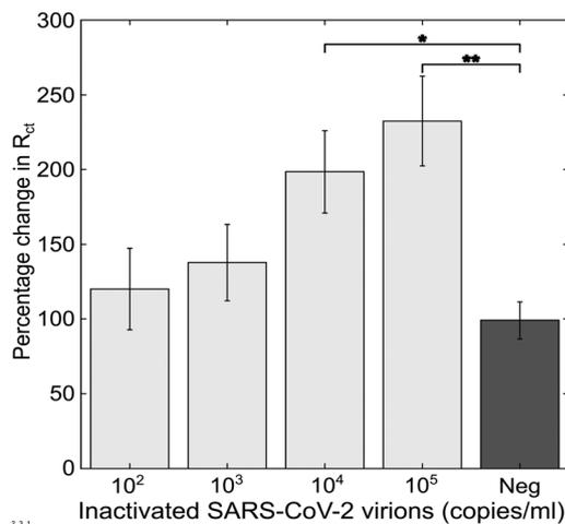
Fig. 2 Dose response following incubation of PFDT-ACE2 modified sensor with inactivated SARS-CoV-2 molecular standards kit. Viral concentration is expressed in copies  $\text{mL}^{-1}$  which is the result of sample quantification following viral inactivation using digital PCR.  $N = 6$  & Error Bars = SE.
