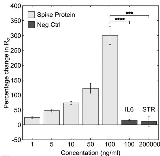
**Fig. 1** Dose response curve for PFDT-ACE2 modified sensors when incubated for 30 min with solutions of recombinant SARS-CoV-2 spike protein. Negative controls: 100 ng mL<sup>-1</sup> IL-6 and 200 μg mL<sup>-1</sup> streptavidin.  $N = 8$  & Error Bars = SE.
