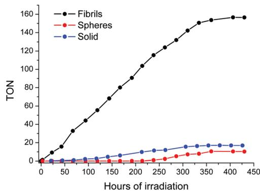
Fig. 5  $\text{H}_2$  evolution plots of **Fmoc-FF-(ZnPor)** upon its self-assembly into spheres (red line), fibrils (black line) and solids (blue line). All the results presented in the  $\text{H}_2$  production plots are the average value of three independent measurements.
