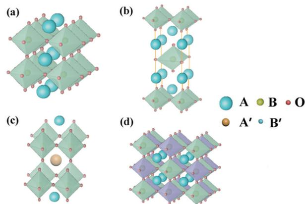
Fig. 3 Crystal structure of (a) the ideal  $ABO_3$ -type perovskite oxides, (b) Ruddlesden–Popper perovskite oxides ( $(AO)(ABO_3)_n$ ), (c) A-site ordered double perovskite oxides ( $AA'B_2O_6$ ) and (d) B-site ordered double perovskite oxides ( $A_2BB'O_6$ ).
