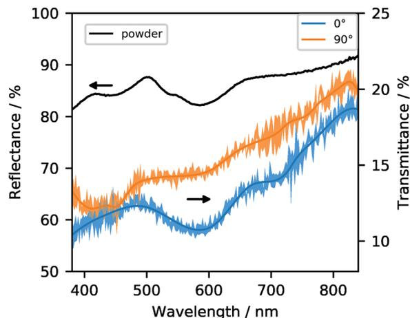
Fig. 3 UV-visible spectra of **1** as powder in diffuse reflectance mode (black) and in single-crystal transmission mode with two relative polarization directions ( $0^\circ$  shown in blue and  $90^\circ$  in orange).<sup>‡</sup> The shaded area corresponds to one standard deviation (see ESI† for details).
