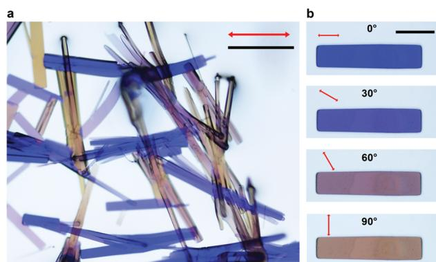
Fig. 2 Optical images of **1**. (a) Various relative orientations with respect to the polarization direction transmit different ranges of visible light. (b) View of an isolated crystal of **1** whose long axis is  $0^\circ$ ,  $30^\circ$ ,  $60^\circ$ , and  $90^\circ$  relative to the polarized light's orientation (red arrows); scale bars are  $200 \mu m$ .
