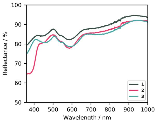
Fig. 4 Diffuse reflectance UV-visible spectra of **1**, **2**, and **3**. Barring the absorption at 375 nm for **2**, the same absorption bands are observed for all frameworks, with slight shifts with respect to **1**.
