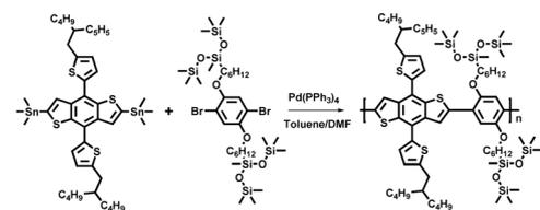
Fig. 5 Synthetic route to P-Si, reagents and conditions.
