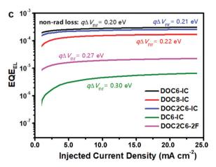
Fig. 14 EQE<sub>EL</sub> of the solar cells based on different acceptors. Copyright 2019, Macmillan Publishers.
