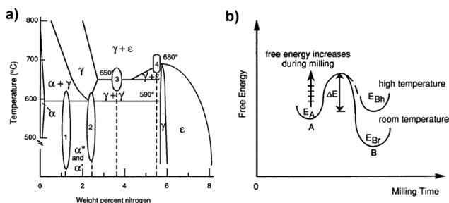
Fig. 6 Nitriding reaction of ball milling anhydrous Fe. (a) Thermal-equilibrium phase diagram of the Fe–N system and (b) schematic of the free-energy changes for ball milled Fe in  $\text{NH}_3$ .<sup>58</sup> Reproduced with permission.<sup>58</sup> Copyright 1996, American Institute of Physics.
