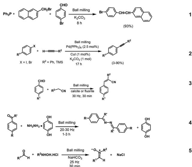
Fig. 5 Various reactions in organic synthesis: (1) one-pot Wittig reaction,<sup>51</sup> (2) Sonogashira reaction,<sup>52</sup> (3) Knoevenagel Condensation,<sup>54</sup> (4) azine formation<sup>55</sup> and (5) nitrene synthesis.<sup>56</sup>
