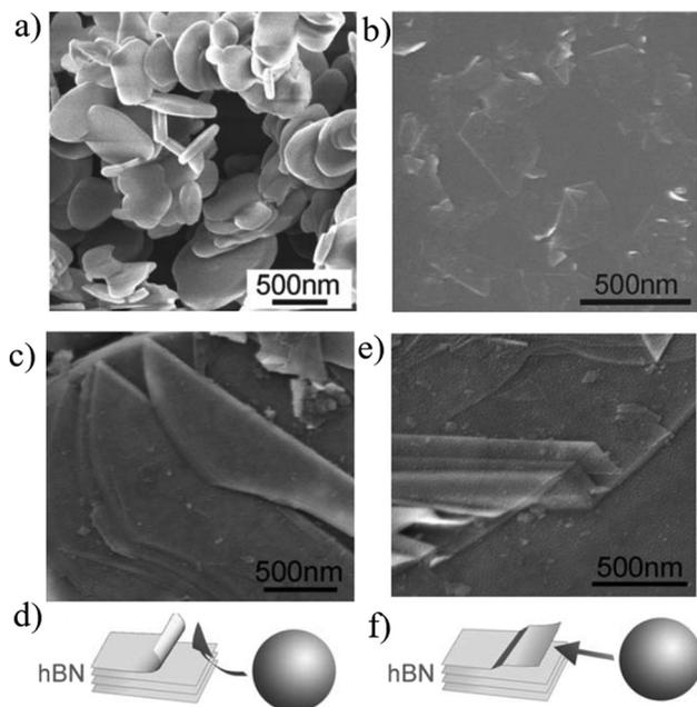
**Fig. 9** SEM images of starting hBN particles: (a) exfoliated BN nanosheets (b); SEM images illustrating the exfoliating mechanisms for peeling off and sliding (c and d), rolling over top and shear force. (e and f) thin sheets peeling off the top surface of an hBN. (a–f) Reproduced with permission.<sup>69</sup> Copyright 2017, Royal Society of Chemistry.
