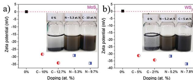
**Fig. 12** Zeta potential of samples milled in  $\text{C}_2\text{H}_4$  and  $\text{NH}_3$ ;  $\text{MoS}_2$  (a) and  $\text{WS}_2$  (b) Reproduced with permission.<sup>71</sup> Copyright 2015, Royal Society of Chemistry.
