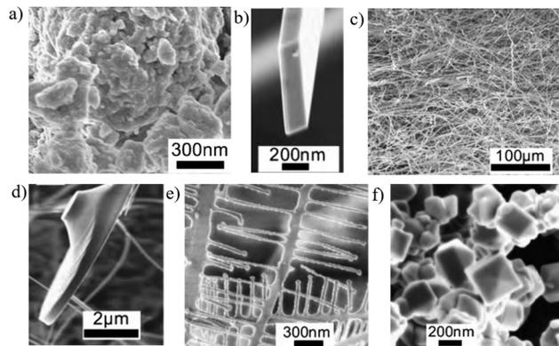
Fig. 8 SEM images of milled and annealed  $\text{SnO}_2$ : (a) milled sample, (b and c) nanoribbons, (d) nanodiskettes (e) nanobranches, (f) nanocrystal. Reproduced with permission.<sup>67</sup> Copyright 2017, Elsevier.
