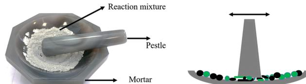
Fig. 1 Traditional method to carry out a chemical reaction with manual grinding.
