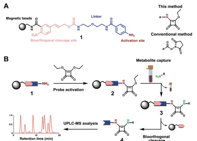
**Fig. 1** Chemoselective probe for amine-containing metabolite analysis. (A) Probe design: magnetic beads (black), bioorthogonal cleavage site (pink), linker (blue), and activation site (red). The reactive moiety for amine capturing is a squaramide ester and the conventional moiety an NHS ester. (B) Chemoselective probe treatment workflow that includes a magnetic separation step of **3** from the sample matrix after incubation.
