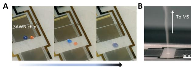
**Fig. 6** On-chip surface acoustic wave nebulization (SAWN). (A) Droplet movements (moving, merging, mixing) on the SAWN chip surface integrated with anisotropic ratchet conveyors (ARCs) pattern. ARCs utilize hydrophilic patterns on a hydrophobic background to control the droplet transport by imbalanced hysteresis force. (B) Droplets nebulization. Adapted from ref. 145 with permission from the Royal Society of Chemistry, copyright © 2020.
