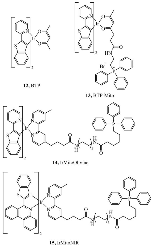
Fig. 4 Cyclometalated Iridium complexes with triphenylphosphine pendants.
