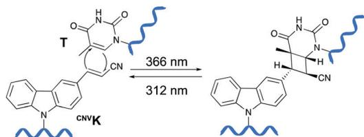
Fig. 5 Mechanism of the photo-crosslinking reaction between 3-cyanovinylcarbazole (<sup>CNVK</sup>) and thymine (T) upon UV-A irradiation (366 nm). Photo-reversibility of the crosslinking reaction can be achieved by irradiating the product at 312 nm.
