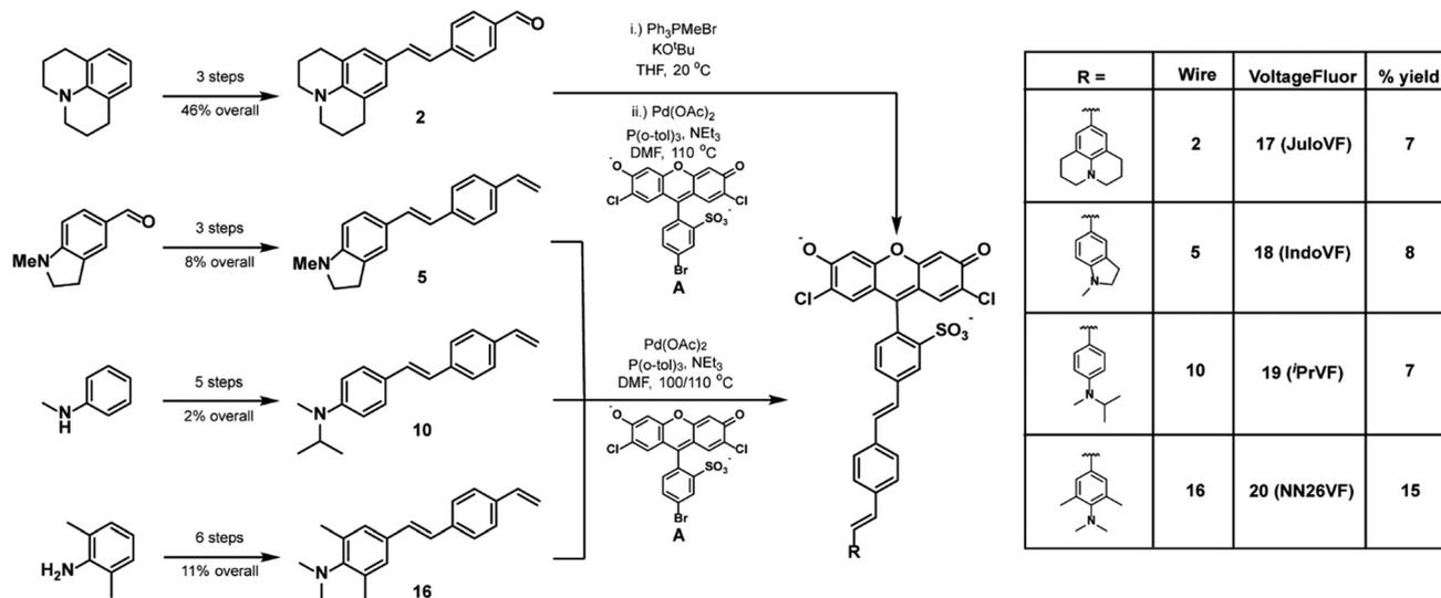
Scheme 2 Synthesis of new VF dye derivatives.
