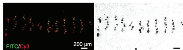
**Fig. 5** Fluorescent and corresponding bright-field images of the cross-section of a dual mixed 3D-printed scaffold. The scaffold labeled with both streptavidin–FITC (green) and DBCO–Cy3 (red) was sectioned to show the homogeneous distribution and colocalization (yellow) of HABind(biotin) and E3(azide) peptides throughout the construct. Bright field images showed both peptides were homogeneously presented throughout the entire construct.
