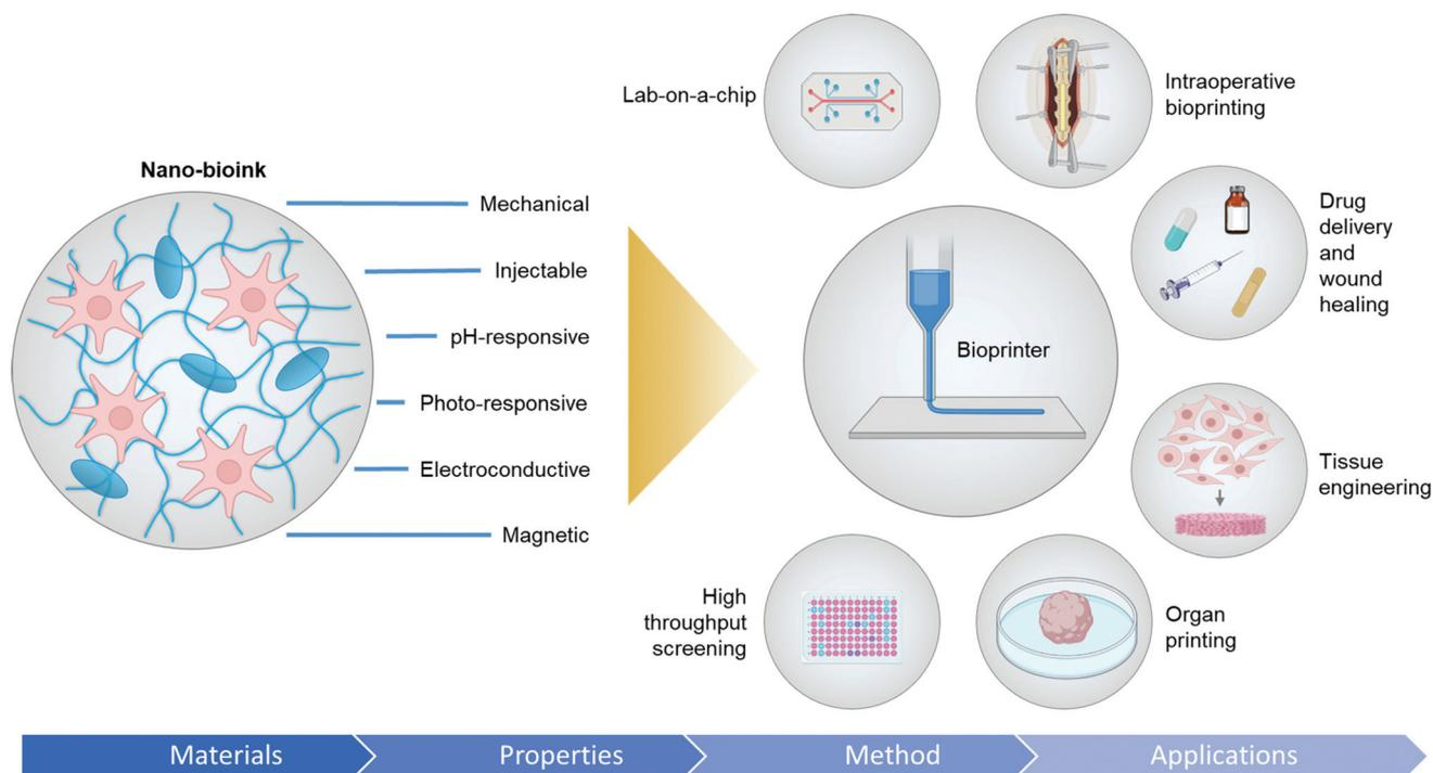
**Fig. 1** Multifunctionalities of nanocomposite hydrogel-based bioinks. Schematic highlights the different functionalities of a bioink imparted by nanoparticles. It also demonstrates the possible applications of nanocomposite hydrogel-based bioinks.
