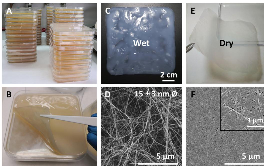
**Fig. 1** BNC synthesis, wet and dry states and microstructure. (A) Numbering up BNC production at laboratory level. (B) A native wet BNC pellicle. (C) Wet form of BNC after cleaning and autoclaving. (D) SEM image of an SC dried BNC sample mimicking the microstructure of a wet BNC film. (E) Dry BNC film. (F) SEM image of the compact nanofiber conformation for dry BNC. Inset: higher magnification to better visualize the nanofibers arrangement.
