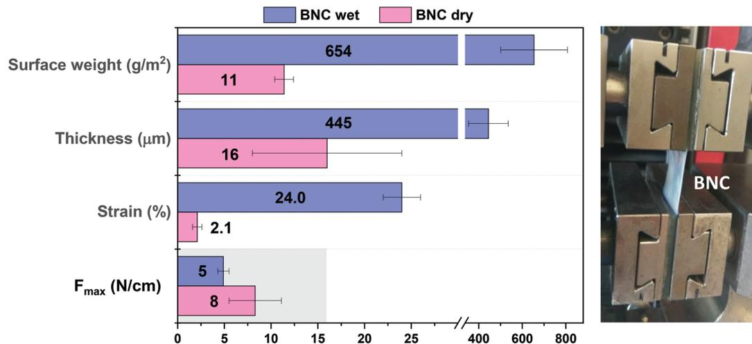
Fig. 2 Mechanical properties of single-layer BNC patches in wet and dry conditions and the experimental setup. Single-layered BNC implants did not meet the acceptance criteria of tensile stress resistance set at  $F_{\max} = 16 \text{ N cm}^{-1}$  (grey area). Statistically significant differences between dry and wet BNC samples were found for all the studied parameters except for the  $F_{\max}$  ( $P$ -values  $< 0.001$ ) ( $n = 5$ ).
