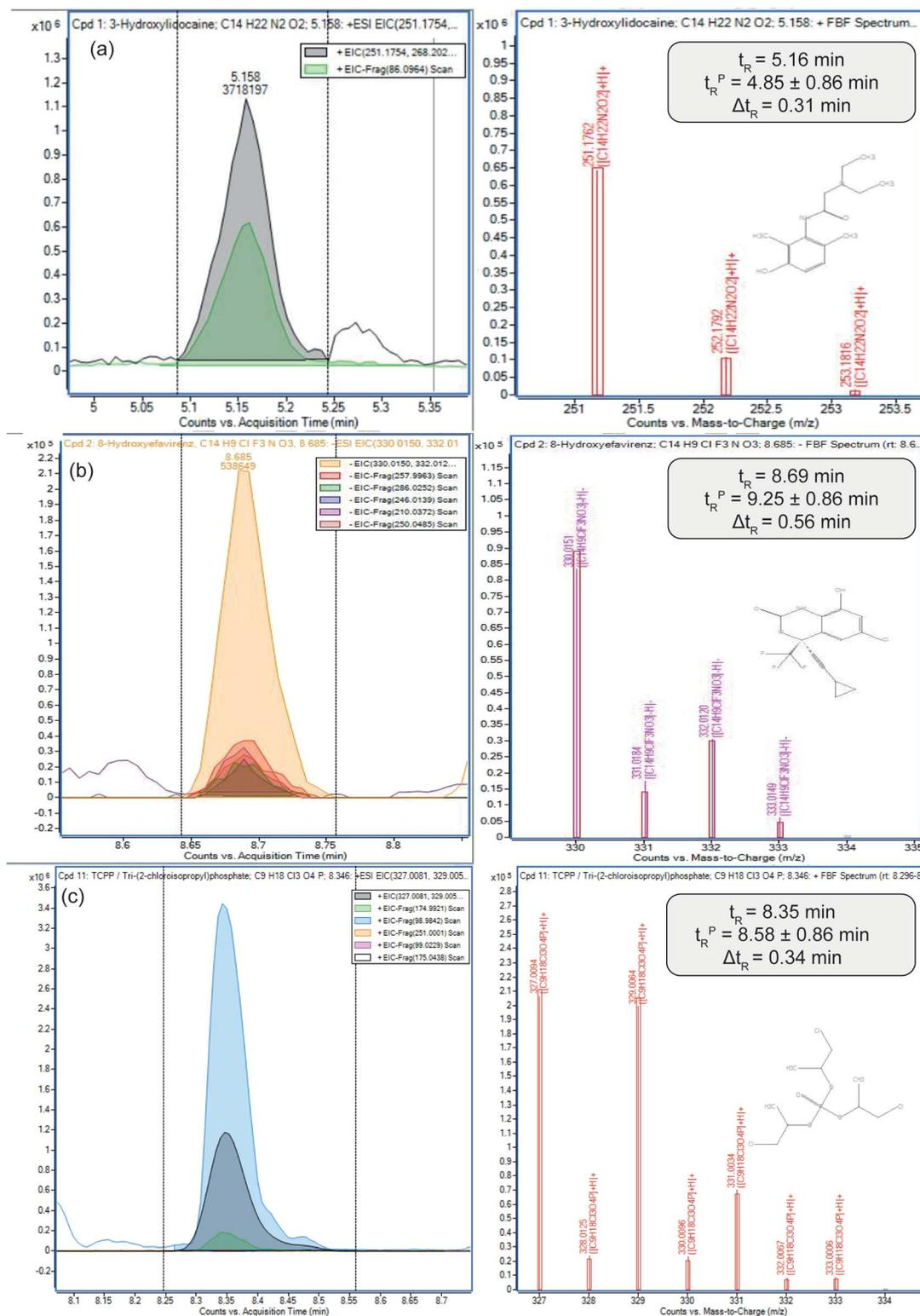
Fig. 3 Extracted ion chromatograms of (a) 3-hydroxyliclocaïne, (b) 8-hydroxyefavirenz and (c) TCPP in the passive sampler extracts. (Left) Extracted ion chromatograms of the  $[M + H]^+$  (a and c) and  $[M - H]^-$  (b) ion and relevant fragments measured by DIA. Right: denotes the isotopic fit of the  $[M + H]^+$  (a and c) and  $[M - H]^-$  (b) and matching predicted retention times.
