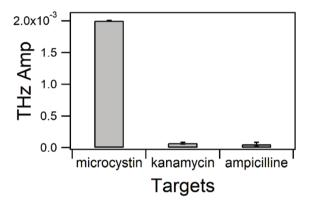
Fig. 6 TCM response to 1  $\mu$ M of MC-LR, kanamycin, and ampicillin. These targets are prepared in the binding buffer that contains 10 mM of Mg<sup>2+</sup> ion concentration. All THz values are presented as means  $\pm$  S.E.M of three trials. The equation  $\sqrt{\Delta X^2 + \Delta Y^2}$  is used to estimate the S.E.M. for each THz value. Here,  $\Delta X$  and  $\Delta Y$  are S.E.M. values for the baseline (buffer) and spiked samples with microcystin, kanamycin, and ampicillin.
