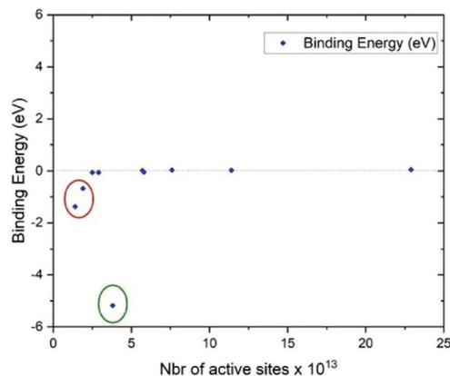
Fig. 3 Calculated binding energy as a function of the AzPTES concentration on the surface ( $\text{SiO}_2$ ). Green circle: optimal concentration, red circle: low concentration.
