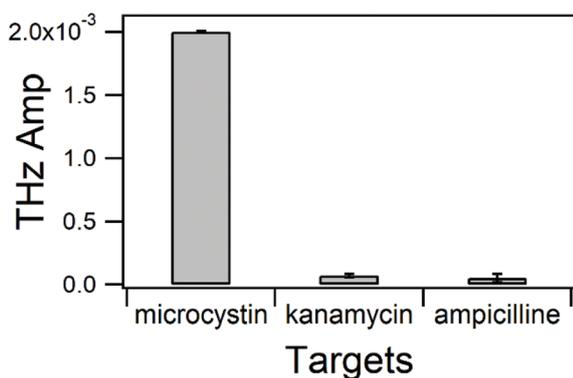
**Fig. 6** TCM response to 1  $\mu$ M of MC-LR, kanamycin, and ampicillin. These targets are prepared in the binding buffer that contains 10 mM of Mg<sup>2+</sup> ion concentration. All THz values are presented as means  $\pm$  S.E.M of three trials. The equation  $\sqrt{\Delta X^2 + \Delta Y^2}$  is used to estimate the S.E.M. for each THz value. Here,  $\Delta X$  and  $\Delta Y$  are S.E.M. values for the baseline (buffer) and spiked samples with microcystin, kanamycin, and ampicillin.
