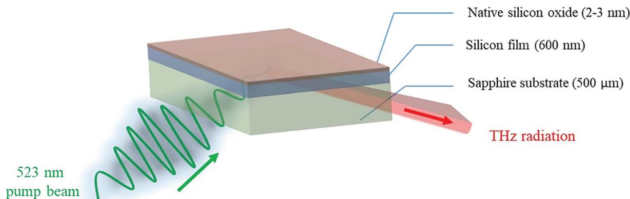
Fig. 1 Schematic diagram showing the composition of the sensing plate and the excitation – detection configuration.
