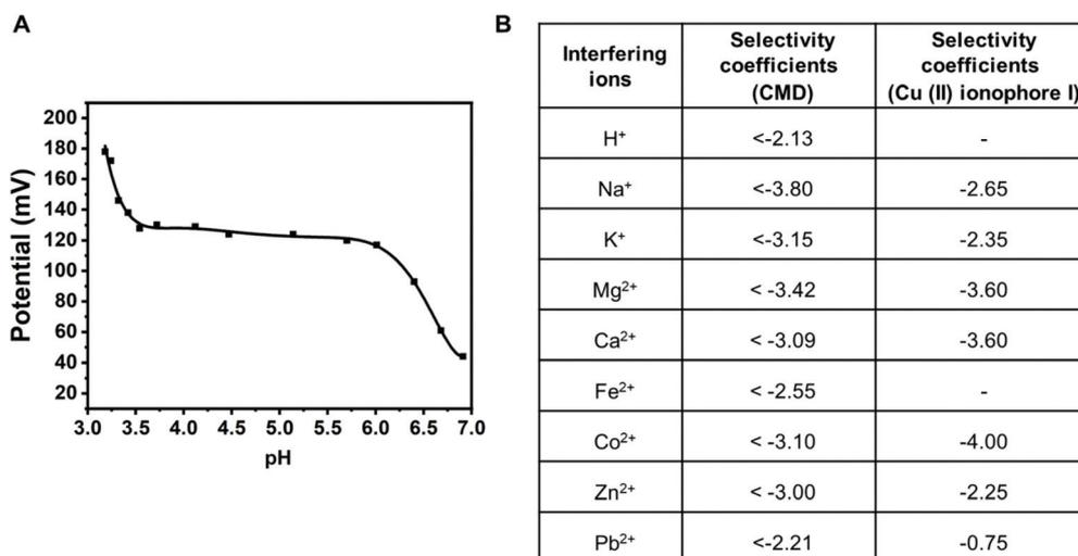
**Fig. 6** (A) Effect of pH on the carbon-packed sensor using the CMD ionophore. (B) The selectivity coefficients table of the carbon-packed sensor using the CMD ionophore is compared against the commercial ionophore (copper(II) ionophore I<sup>51</sup>). The selectivity coefficients for both the ionophores were obtained using the fixed interference method.
