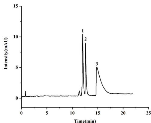
**Fig. 5** (a) Separation behavior of food additives on the TzDa@capillary. Experimental conditions: mobile phase, 20% methanol in pH 9.0 30 mM phosphate buffer; applied voltage, 20 kV; injection, 15 mbar  $\times$  5 s; detection wavelength, 210 nm. Peaks: 1, vanillin; 2, isovanillin; 3, eugenol.
