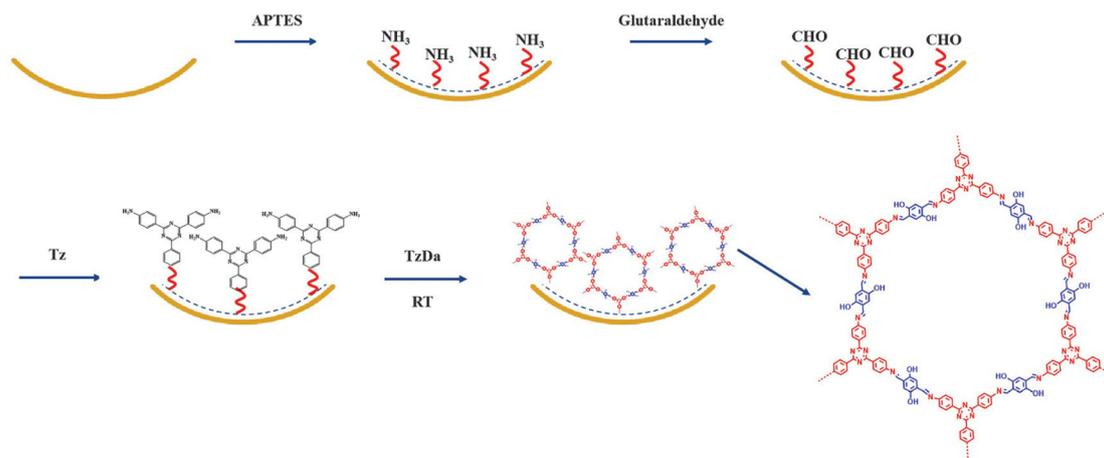
Fig. 1 Schematic procedure for the fabrication of the TzDa@capillary.
