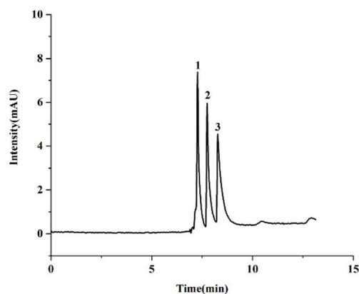
**Fig. 4** Separation behavior of phenolic compounds on the TzDa@capillary. Experimental conditions: mobile phase, 25% ACN in pH 9.0 30 mM phosphate buffer; applied voltage, 20 kV; injection, 7 mbar  $\times$  5 s; detection wavelength, 230 nm. Peaks: 1, hydroquinone; 2, resorcinol; 3, catechol.
