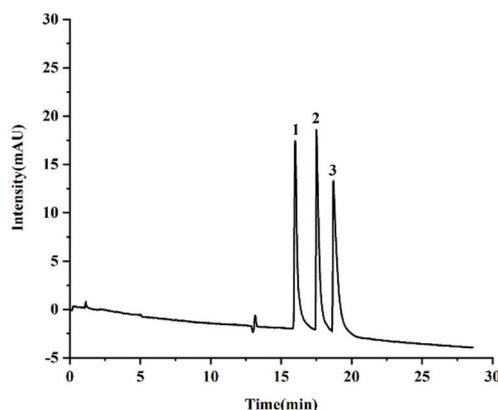
**Fig. 6** Separation behavior of amino acids on the TzDa@capillary. Experimental conditions: mobile phase, 40% methanol in pH 8.0 20 mM phosphate buffer; applied voltage, 20 kV; injection, 25 mbar  $\times$  5 s; detection wavelength, 210 nm. Peaks: 1, tryptophan; 2, tyrosine; 3, phenylalanine.
