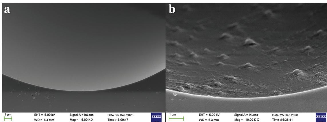
Fig. 2 SEM images of the inner wall of the bare capillary (a, 5000 $\times$ ) and the TzDa@capillary (b, 10 000 $\times$ ).
