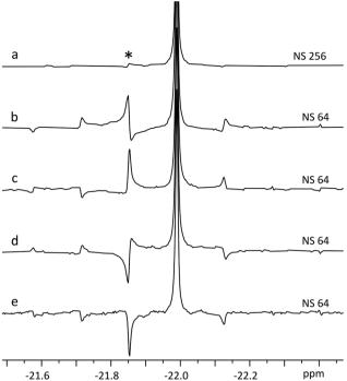
**Fig. 5** Fourier transform after LP of four SAPPHIRE experiments (b–e) on ATP  $\beta$ -phosphate (20 mM). Note how the artefacts are pairwise in opposite phases in traces b  $\vartheta$  d and c  $\vartheta$  e. Trace (a) displays FT of the sum of FID-s from b–e, where the chunking artefacts have been largely cancelled out, <sup>20</sup> with the most prominent artefact (\*) having <2% intensity of the main signal.
