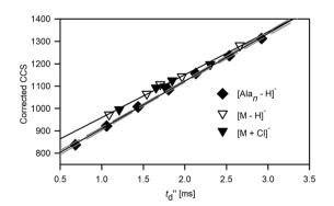
Fig. 4 Relationship between the calibration plots (N<sub>2</sub>) for deprotonated polyalanine ions (Ala<sub>n</sub>, n = 4-10) and macrocyclic ions:  $[M - H]^{-}$  and [M+ Cl] obtained for N<sub>2</sub> drift gas (recorded at ratios of traveling wave velocity [m s $^{-1}$ ] to wave height [V]: 350/29). The 95% confidence bands for the polyalanine plot are shown.
