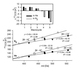
Fig. 1 Relationship between m/z and  ${}^{\rm DT}{\rm CCS}_{{\rm He/N_2}}$  values obtained from direct measurements of deprotonated macrocycles [M - H]- (open symbols) and macrocyclic complexes with Cl<sup>-</sup> (black symbols). The top part shows the directions of the CCS shifts upon Cl<sup>-</sup> complexation.
