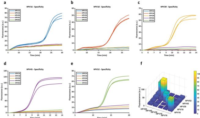
Fig. 4 Evaluation of the specificity of the microfluidic detection system. Cross-reactivity tests for (a) HPV16; (b) HPV18; (c) HPV39; (d) HPV45; and (e) HPV52. (f) Histogram overview of specificity analysis.
