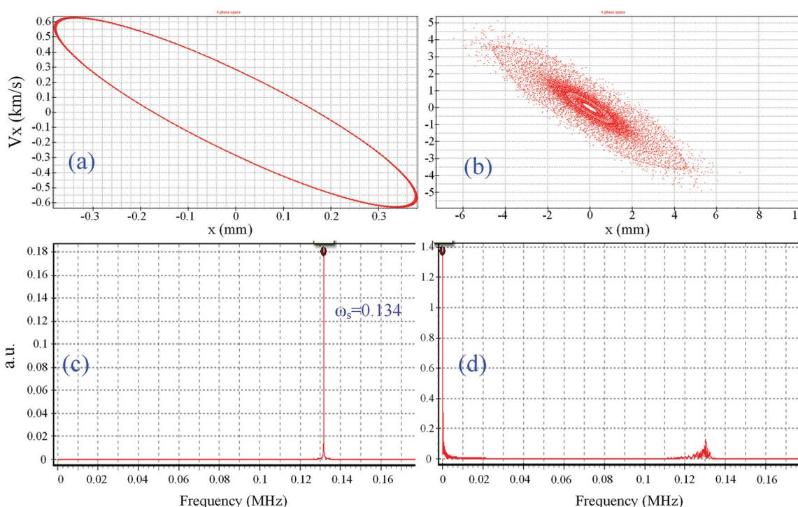
**Fig. 5** (a) The simulating  $x$  phase space in the ion trap in the  $x$ -direction when there is no AC. (b) The simulating  $x$  phase space in the ion trap on the  $x$ -direction when there is AC. (c) The simulative frequency spectra of reserpine in the cRIT when there is no AC. (d) The simulative frequency spectra of reserpine in the cRIT when there is AC.
