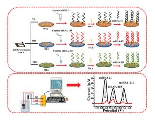
Fig. 1 The diagram of AuNPs/GQDs/GO-based biosensors for the detection of miRNA-21, miRNA-155, and miRNA-210 related to breast
