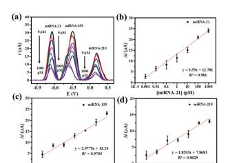
Fig. 5 (a) SWV responses of the proposed biosensor after incubation with different concentrations of miRNA-21, miRNA-155, and miRNA-210, and (b), (c) and (d) corresponding calibration curves of the triplet assay towards miRNA-21, miRNA-155, and miRNA-210 respectively, in 10 mM PBS solution (pH 7.4).
