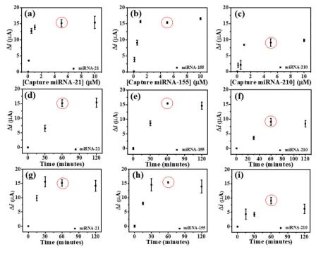
Fig. 4 The influence of (a) capture miRNA-21 probe concentration, (b) capture miRNA-155 probe concentration, and (c) capture miRNA-210 probe concentration, anchoring time for (d) capture miRNA-21 probe, (e) capture miRNA-155 probe, (f) capture miRNA-210 probe, and hybridization time on the detection of (g) miRNA-21, (h) miRNA-155 and (i) miRNA-210 using the AuNPs/GQDs/GO/SPCE-based biosensor.
