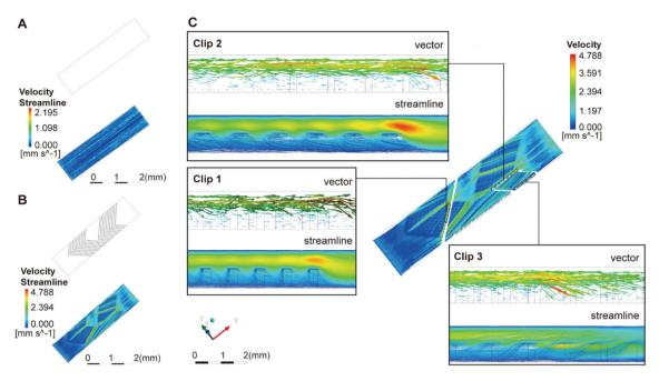
Fig. 2 Simulation of flow in the microfluidic chip. The flow field morphology observed from (A) a straight microchannel without herringbones, (B) a straight microchannel with herringbones, and (C) three clips on the microchannel with herringbones including the streamline and vector plots.
