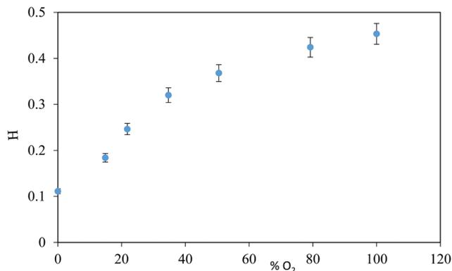
Fig. 2 Sensor response to O<sub>2</sub>.
