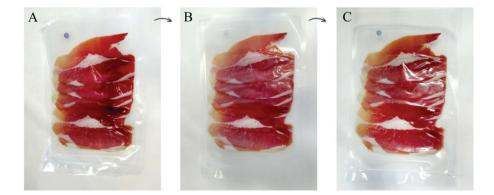
Fig. 5 Photographs of UVA-activated oxygen indicator placed inside a plastic package flushed with CO2 and sealed: (A) the package is recently sealed and the indicator is blue; (B) the indicator has been bleached by a UVC light burst, the indicator inside remains bleached for 48 h; and (C) upon opening the package, the entrance of oxygen causes the indicator to recover its original colour.
