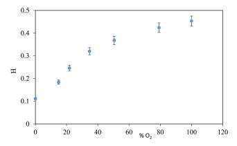
Fig. 2 Sensor response to O<sub>2</sub>.
