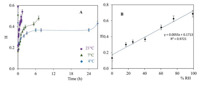
Fig. 3 Influence of sensor response to experimental variables: (A) influence of temperature; and (B) influence of % RH.
