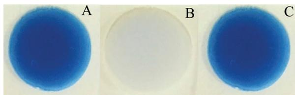
**Fig. 1** Images of the printed sensor: (A) before UVA irradiation; (B) immediately after irradiation; and (C) sometime after exposure to oxygen (in air) when it has fully recovered its original colour.
