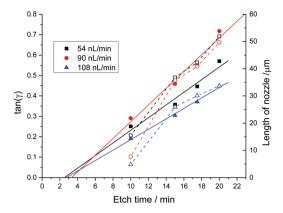
Fig. 3 Dependence of the axicon angle,  $\gamma$ , (solid symbols with solid linear fit line) and the nozzle length (empty symbols) on the flow rate of water through the channels and on the etch time in HF-solution. The post angle,  $\alpha$ , remained unchanged at 68.7  $\pm$  1.3 degrees for all etch times and flow rates.
