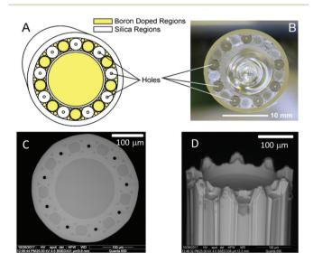
Fig. 1 Illustration of the MSF fabrication process. A fiber preform shown schematically in (A) was prepared by stacking silica and borosilica rods and tubes in a carefully designed pattern. The preform (B) was then drawn into an MSF. Panel (C) shows the cleaved MSF and (D) shows the MSF after etching in hydrofluoric acid solution.
