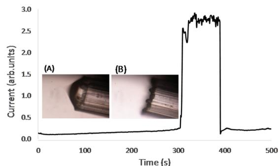
**Fig. 6** Spray current for an emitter etched at a flow rate of 54  $\text{nL min}^{-1}$  for 20 minutes. Emission from a single Taylor cone (A) is observed except between 300 s and 400 s where nine Taylor cones are formed in front of each nozzle (B). The flow rate is 800  $\text{nL min}^{-1}$ .
