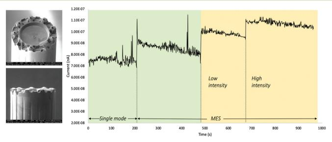
Fig. 7 (Left) SEM images of a MES emitter, which was etched for 12.5 minutes at a water flow rate of 90 nL  $\min^{-1}$ . The resulting micronozzles have an axicon angle of 15 degrees and 29 µm nozzle length. (Right) Spray current acquired with the class IIIB laser off (green) and on (yellow). The data indicate that different laser conditions (i.e. high or low intensity) and electrospray modes (single or MES) result in different desolvation efficiencies and consequent ion current.
