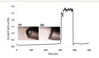
Fig. 6 Spray current for an emitter etched at a flow rate of 54 nL min<sup>-1</sup> for 20 minutes. Emission from a single Taylor cone (A) is observed except between 300 s and 400 s where nine Taylor cones are formed in front of each nozzle (B). The flow rate is 800 nL min<sup>-1</sup>.
