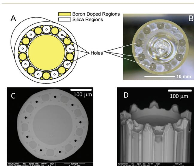
**Fig. 1** Illustration of the MSF fabrication process. A fiber preform shown schematically in (A) was prepared by stacking silica and borosilicate rods and tubes in a carefully designed pattern. The preform (B) was then drawn into an MSF. Panel (C) shows the cleaved MSF and (D) shows the MSF after etching in hydrofluoric acid solution.
