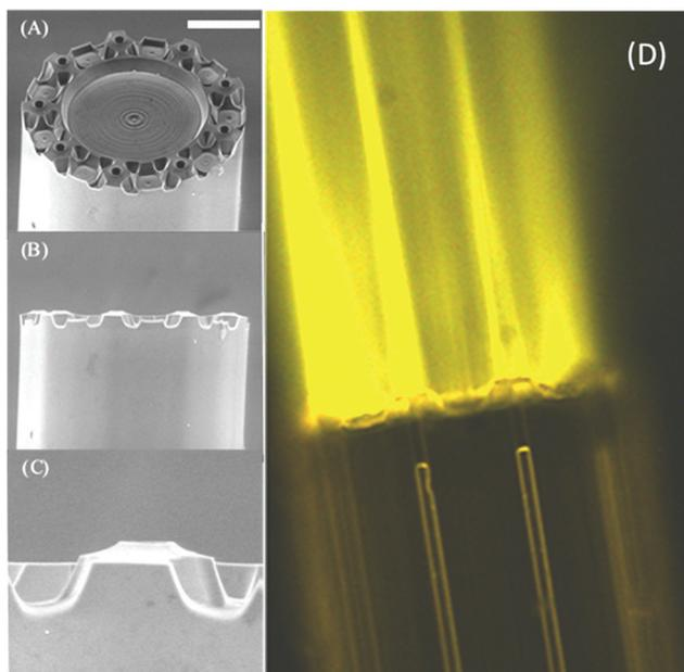
**Fig. 4** (A)–(C) SEM images of the MES emitter illustrating the nozzle and facet profile. (D) Optical microscope image depicting the fluorescence intensity distribution for the emitter illuminated with 532 nm radiation and submerged in a fluorescent solution of rhodamine 6G dye. White scale bar is 100  $\mu\text{m}$ .
