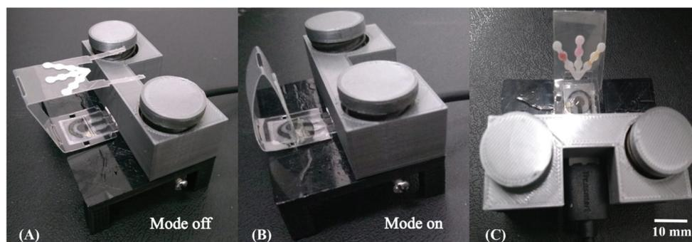
**Fig. 3** Schematic view of the 3D printed holder integrating both  $\mu$ PAD and ePAD through vertical folding assembly. Images (A) and (B) show the assembling of the multiplexed device before (mode off) and after (mode on) coupling, respectively. Image (C) depicts the disconnected  $\mu$ PAD after colorimetric assays enabling the use of ePAD for metal analysis using the same sample aliquot.
