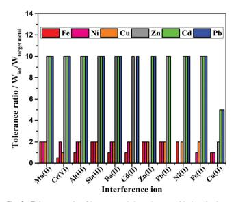
Fig. 6 Tolerance ratio of heavy metal detection considering the interference ion  $\leq$ 10%, using target metals solutions of 500  $\mu$ g L<sup>-1</sup> for Zn( $\shortparallel$ ), Cd( $\shortparallel$ ), Pb( $\shortparallel$ ) and 5.0 mg L<sup>-1</sup> for Fe( $\iota$ ), Ni( $\iota$ ), Cu( $\iota$ ).
