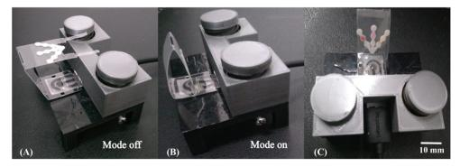
Fig. 3 Schematic view of the 3D printed holder integrating both µPAD and ePAD through vertical folding assembly. Images (A) and (B) show the assembling of the multiplexed device before (mode off) and after (mode on) coupling, respectively. Image (C) depicts the disconnected µPAD after colorimetric assays enabling the use of ePAD for metal analysis using the same sample aliquot.
