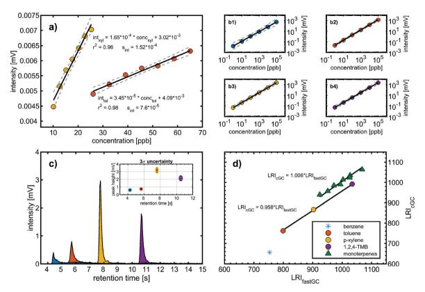
Fig. 2 Analytical figures of merit comprising (a) calibration functions of toluene (T) and p-xylene (X) with a coefficient of determination  $r^2$  and residual standard deviation  $s_{int}$ , (b1-b4) linearity over five orders of magnitude, (c) peak shape and precision (3 $\sigma$ ) of intensity and retention time from repeated BTXT analysis, and (d) comparison of the LRI obtained from fastGC with the LRI obtained from cGC for BTXT and 8 monoterpenes.
