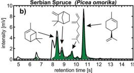
Fig. 3 Chromatogram of the headspace analysis of needles from (a) black pine and (b) Serbian spruce. The black line denotes the total ion intensity, while the green area represents the monoterpene-related ion intensities m/z 80, 92, 93, 94, 107 and 121, and the molecular ion at m/z136
