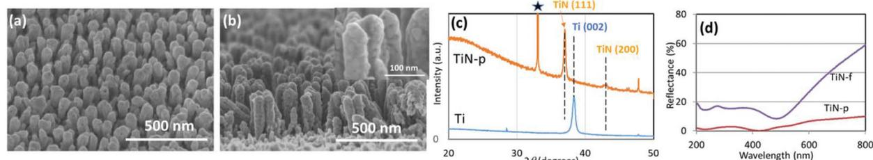
**Fig. 1** Characterizations of TiN-p. SEM images showing (a) a tilted top view and (b) a cross-sectional view. The inset in (b) shows a magnified image. (c) XRD pattern of TiN-p; the profile of the Ti film is shown for comparison. The peak marked with an asterisk corresponds to Si (002) of the silicon substrate. (d) Reflectance spectra of TiN-f and TiN-p.
