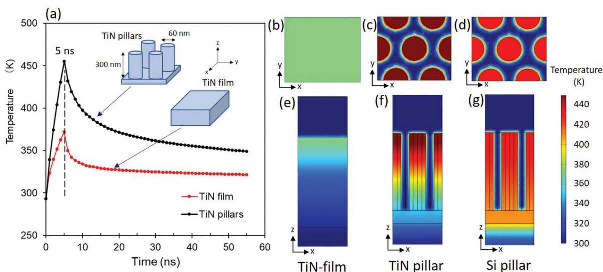
**Fig. 8** Theoretical heat-transfer modeling. (a) Temperatures of the top surfaces of the TiN film and the TiN pillars as functions of time after irradiation with an electromagnetic wave (355 nm, 5 ns). (b–g) Temperature distributions in the (b–d)  $xy$  and (e–g)  $xz$  planes after irradiating (b, e) the TiN film, (c, f) the TiN pillar, and (d, g) the Si pillar for 5 ns.
