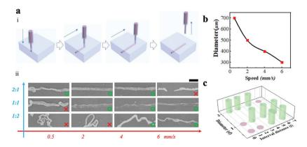
Fig. 2 (a) Schematic diagram of 3D printing (i) and printing performance under different nozzle moving speeds and PVA: SF ratios; scale bar: 0.5 cm (ii); (b) relationship between the printing speed and printing diameter. (c) Diagram of printing performance (i), red: non-printable; green: printable.
