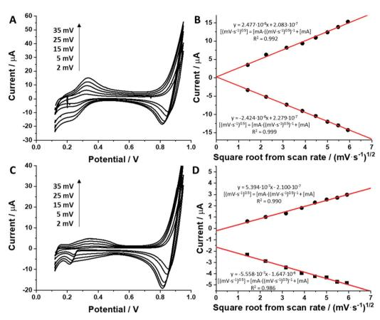
Fig. 4 A and C are ion transfer voltammograms recorded at 2; 5; 15; 25 and 35 mV s<sup>-1</sup>, whereas B and D show current *versus* square root of the scan rate dependency. Graphs A and B correspond to the BDTR-2 (100 μM) dendrimer. Graphs C and D correspond to the BDTR-5 dendrimer (50 μm). Linear fit equations are displayed next to the corresponding experimental data points.
