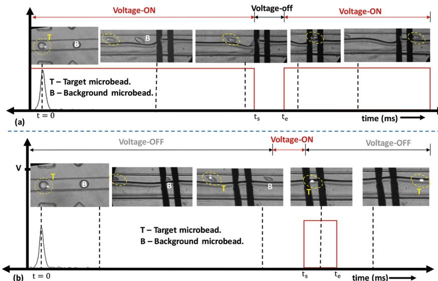
**Fig. 5** Experimental images showing the time evolution of target droplets (T) that contain FL microbeads and background droplets (B) that contain non-FL microbeads in the detection and electro-coalescence regions, and the ON/OFF control of the electrode voltage: (a) positive sorting and (b) negative sorting.
