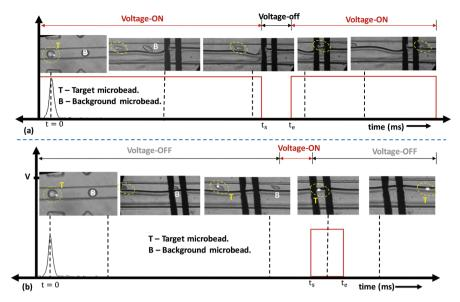
Fig. 5 Experimental images showing the time evolution of target droplets (T) that contain FL microbeads and background droplets (B) that contain non-FL microbeads in the detection and electro-coalescence regions, and the ON/OFF control of the electrode voltage: (a) positive sorting and (b) negative sorting.
