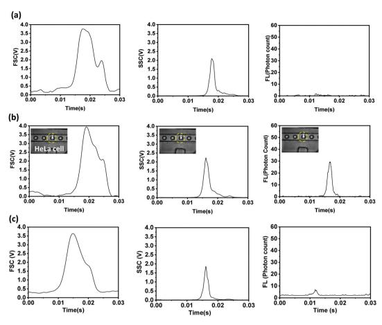
Fig. 3 The FSC, SSC, and FL signals collected from 68 μm droplets encapsulating (a) non-fluorescent, and fluorescent (b) R6G-tagged and (c) anti-Ep-CAM-FITC-tagged HeLa cells.
