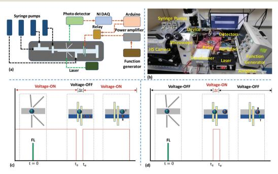
Fig. 2 (a) A schematic diagram of the experimental setup, (b) a photograph of the experimental setup, and the time evolution of the detection and electro-coalescence-based sorting of target cells from background cells in (c) positive and (d) negative sorting modes.
