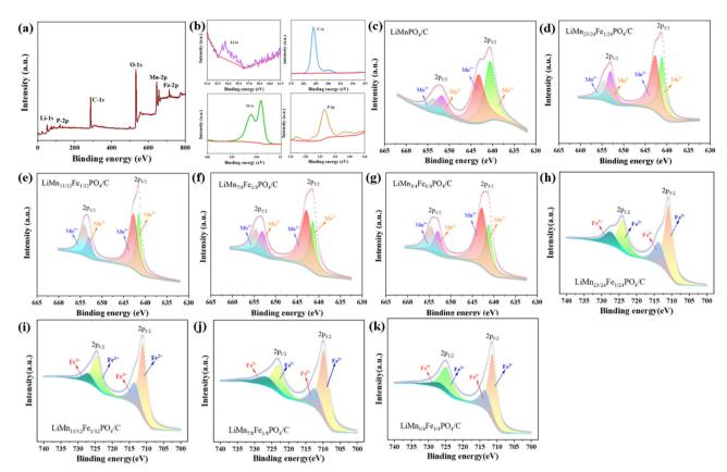
Fig. 5 XPS spectra of LiMn<sub>3/4</sub>Fe<sub>1/4</sub>PO<sub>4</sub>/C composites: (a) total energy spectrum; (b) the Li element in the 1s orbital, the C element in the 1s orbital, the P element in the 2p orbital and the O element in the 1s orbital; (c)–(g) Mn 2p orbital XPS profiles of the  $Li(Mn_{1-x}Fe_x)PO_4/C$  sample; (h)–(k) Fe 2p orbital XPS profiles of the Li( $Mn_{1-x}Fe_x$ )PO<sub>4</sub>/C sample.
