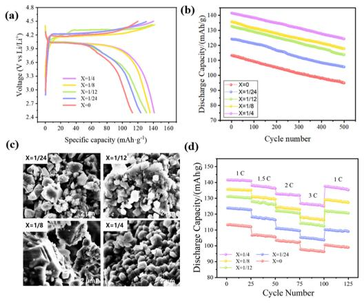
Fig. 8 (a) The initial charge and discharge curves of Li(Mn<sub>1-x</sub>Fe<sub>x</sub>)PO<sub>4</sub>/C at 1C. (b) The cycling performance of the Li(Mn<sub>1-x</sub>Fe<sub>x</sub>)PO<sub>4</sub>/C sample at 1C. (c) SEM images of  $Li(Mn_{1-x}Fe_x)PO_4/C$  after 500 cycles. (d) The rate capability of the  $Li(Mn_{1-x}Fe_x)PO_4/C$  sample.
