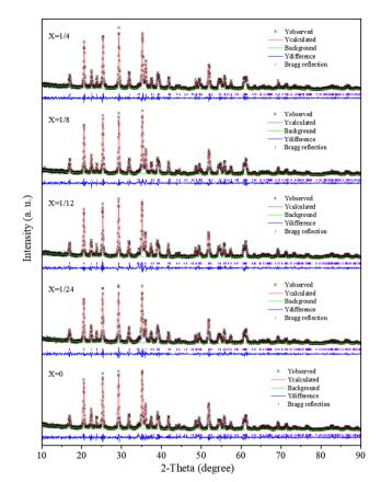
Fig. 4 The Rietveld patterns of Li(Mn<sub>1-x</sub>Fe<sub>x</sub>)PO<sub>4</sub>/C materials.
