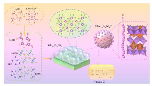
Fig. 2 The plot of the Li(Mn<sub>1-x</sub>Fe<sub>x</sub>)PO<sub>4</sub>/C (x = 0, 1/24, 1/12, 1/8, 1/4) composite material.
