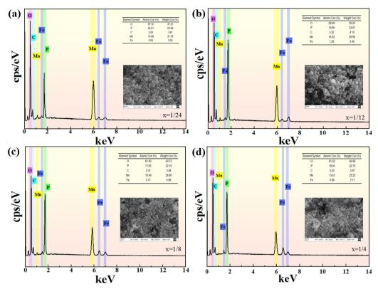
Fig. 6 The SEM images and EDS spectra of Li(Mn<sub>1-x</sub>Fe<sub>x</sub>)PO<sub>4</sub>/C
