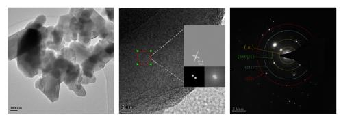
Fig. 7 (a) TEM image, (b) HRTEM image, and (c) SAED pattern of LiMn<sub>3/4</sub>Fe<sub>1/4</sub>PO<sub>4</sub>/C cathode materials.
