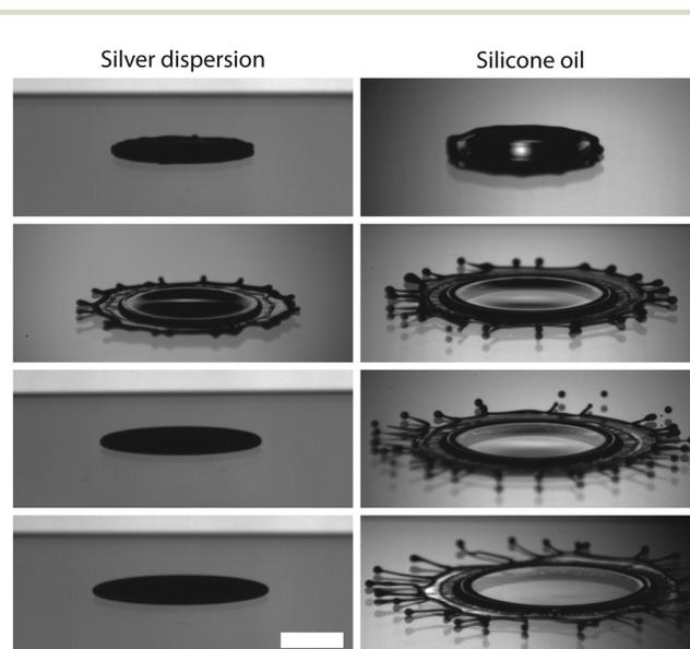
Fig. 1 Comparison of the splashing dynamics of the SA silver dispersion (left,  $We = 216, 511, 604, 1263$ ,  $D = 1.82$  mm) with a silicone oil of similar material properties  $\mu = 9.35$  mPa s and  $\sigma = 20.1$  mN m<sup>-1</sup> (right,  $We = 164, 463, 555, 1169$ ,  $D = 2.03$  mm). The scale bar is 2 mm, same for all panels.
