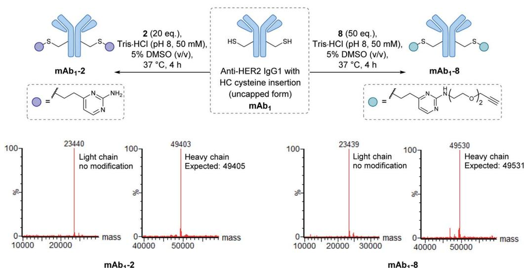
Fig. 4 The modification of **mAb<sub>1</sub>** with linker **2** and **8**. The samples were deglycosylated and reduced prior to LCMS analysis.
