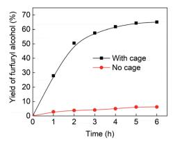
Fig. 4 Yields of furfuryl alcohol *vs.* time in the presence of 9 mol% cage (black line and squares) or in the absence of cage (red line and circles). Yields in the presence of cage are isolated yields. Yields in the absence of cage were determined by <sup>1</sup>H NMR and are likely to be slight overestimates of the amount of furfuryl alcohol produced.
