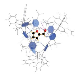
Fig. 2 Calculated orientation of the furfural substrate within the Fe<sub>4</sub>L<sub>6</sub> cage. Dashed lines depict the two hydrogen bond types that anchor the substrate in the cage: CH··· $\pi$  interactions with the aromatic rings of the cage ligands (blue); and O···H–C interactions with the carbonyl group projected towards a triangular opening in the wall of the cage (magenta).
