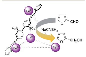
Scheme 1 An illustration of the general class of reactions explored in this work, using the example of furfural reduction to furfuryl alcohol using sodium cyanoborohydride (NaCNBH<sub>3</sub>) as the reducing agent. Only one of the six identical edges of the anionic  $Fe_4^{II}L_6$  cage is shown for clarity.
