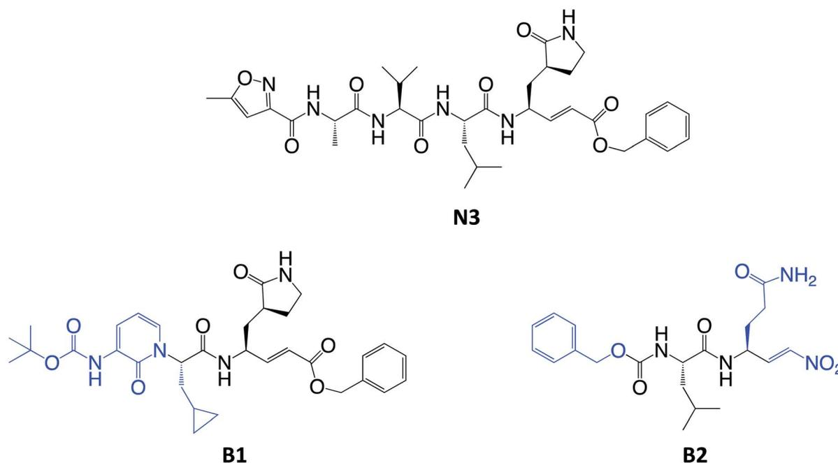
**Scheme 2** Chemical structures of known (N3) and proposed (B1 and B2) Michael acceptor inhibitors of SARS-CoV-2 M<sup>Pro</sup>. The modifications from N3 to B1 and B2 are highlighted in blue.
