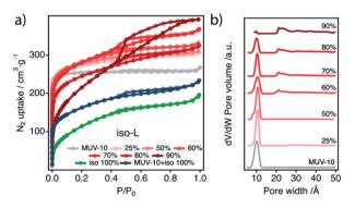
Fig. 8 (a)  $N_2$  adsorption (filled) and desorption (empty symbols) isotherms at 77 K of the iso-L samples, the iso 100% phase and a physical mixture of MUV-10 and the iso 100% phase (50% by weight). (b) PSD of the iso-L series showing the onset of mesoporosity for increasing concentrations of the modulator as calculated with NLDFT by using the QSDT cylindrical pore oxide surface model.
