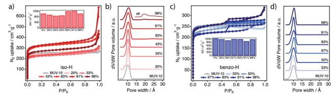
Fig. 7 N<sub>2</sub> adsorption (filled symbol) and desorption (empty symbol) isotherms at 77 K of the series (a) iso-H and (c) benzo-H showing the progressive changes in the uptake profile and surface area with the concentration of the modulator used. (b and d) Changes in the pore size distributions (PSDs) for both sets as calculated by using nonlinear solid density functional theory (NLDFT) by assuming the QSDT cylindrical pore oxide surface model.
