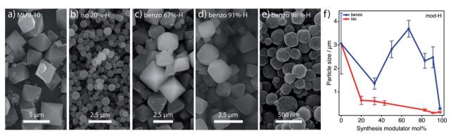
Fig. 6 SEM pictures comparing the changes in size and morphology of (a) pristine MUV-10, (b) iso 20%-H and benzo-H: (c) 67%, (d) 91% and (e) 98%. (f) Evolution of the particle size as a function of the concentration of the modulator in the H region as estimated from the digital analysis of the SEM images. Error bars stand for the calculated standard deviation.
