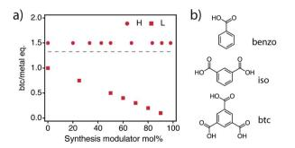
Fig. 3 (a) Synthetic sets designed to study the impact of modulators on the promotion of defects for fixed and variable amounts of btc/metal ratios above (H) and below (L) the stoichiometric ratio fixed by the formula of MUV-10 (dashed line). (b) Modulators with increasing denticity used in this study and the linker btc.
