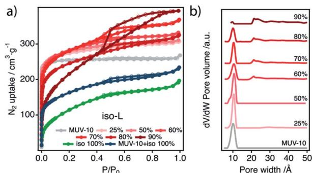
Fig. 8 (a) N<sub>2</sub> adsorption (filled) and desorption (empty symbols) isotherms at 77 K of the iso-L samples, the iso 100% phase and a physical mixture of MUV-10 and the iso 100% phase (50% by weight). (b) PSD of the iso-L series showing the onset of mesoporosity for increasing concentrations of the modulator as calculated with NLDFT by using the QSDT cylindrical pore oxide surface model.
