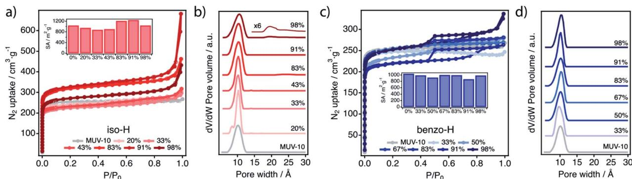
Fig. 7  $N_2$  adsorption (filled symbol) and desorption (empty symbol) isotherms at 77 K of the series (a) iso-H and (c) benzo-H showing the progressive changes in the uptake profile and surface area with the concentration of the modulator used. (b and d) Changes in the pore size distributions (PSDs) for both sets as calculated by using nonlinear solid density functional theory (NLDFT) by assuming the QSDT cylindrical pore oxide surface model.
