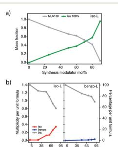
Fig. 5 (a) Variation of the relative fraction of MUV-10 and iso-100% phases for increasing concentrations of isophthalic acid as estimated from a combination of EDX and TG analysis. (b) Comparison of the amount of btc, isophthalic and benzoic acid in the framework in the L regions for increasing concentrations of the modulator.
