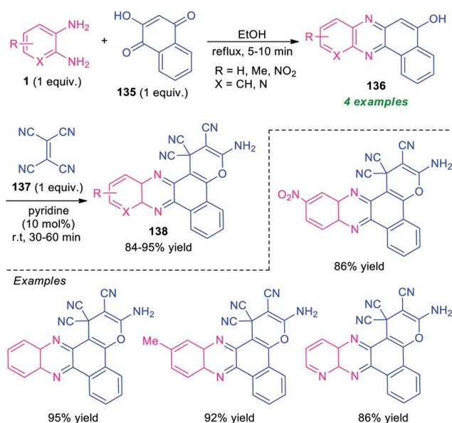
Scheme 40 One-pot two-step three-component synthesis of pyrano-fused quinoxalines.
