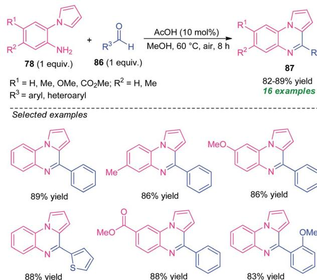
Scheme 28 Acetic acid-catalyzed efficient synthesis of pyrrolo[1,2-*a*]quinoxalines through Pictet–Spengler reaction.
