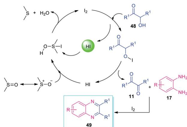
Scheme 14 Iodine catalyzed one-pot oxidation/cyclization to access quinoxalines **49**.
