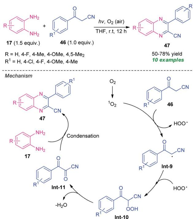
Scheme 13 Visible light-induced electron-transfer and oxidative cyclization to access quinoxaline derivatives.
